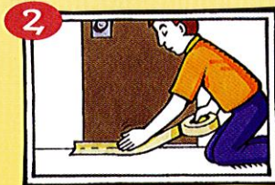
Tape off doorways and edges.
